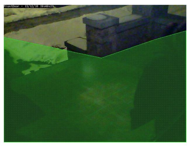
The sample region shown to the right shows a region defined by 6 control points. The shape of the region causes the check methods to ignore the sidewalk and areas of the porch wall that receive changing sunlight; two conditions that are not of interest in this zone.
